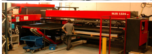
Stansing – fullautomatisert revolver.
